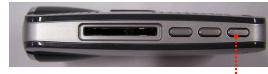
Push "▼" button for 3 sec for Self Format
