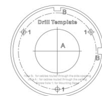
Figure 2-4 Drill Template of Junction Box
