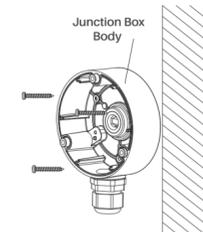
Figure 2-6 Secure the Junction Box on the Wall/Ceiling
